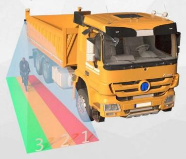
\*Support BSD cam installed back or front / dual BSD, max 4BSD supported.
